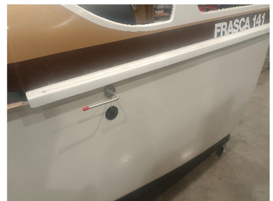
Figure 6 Frasca pitot tube and static port installation
