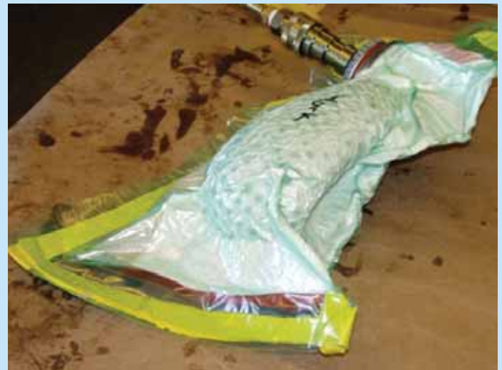
Figure 8. Main gear wheel pant under vacuum
