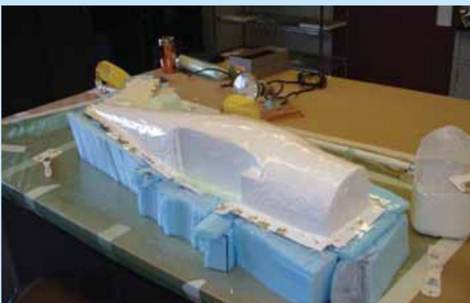
Figure 4. Epoxy Surface Coat applied to the first half of plug
