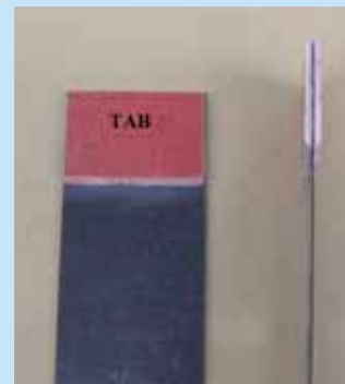
Figure 4. The tabs fixed to the end of the test strips.
