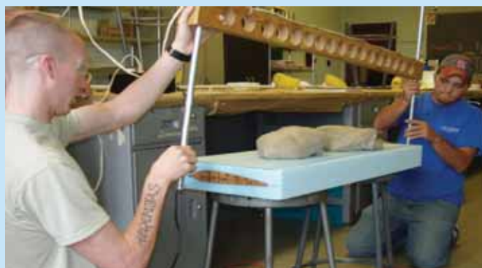
Figure 7. Students using hot wire to cut wing foam core
