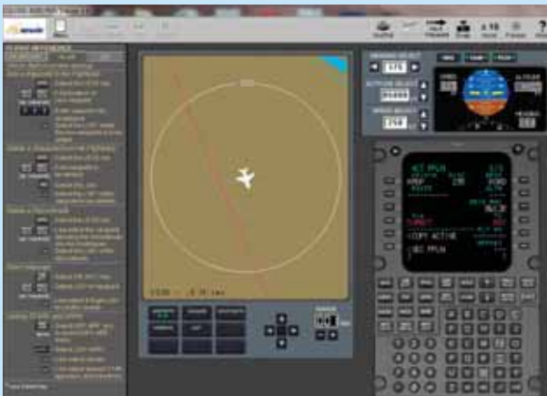
Aerosim's Collins 4200 FMS layout
